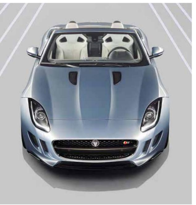
In addition to the structural alloy, Jaguar further developed a skin panel alloy in order to deliver the desired design language. This AC600 alloy offers the same robustness and quality of finish as the existing metal used on the XK but with much greater formability to provide greater clarity and tightness of radii and feature lines.
